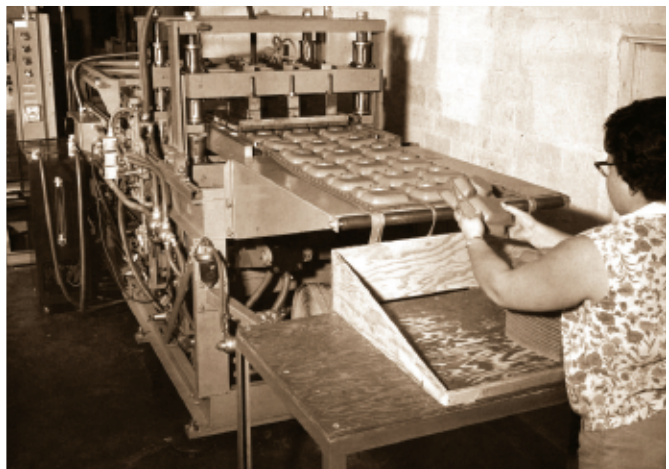
Frito Lay Sip 'n Dip trays are being made on the first new pressure forming machine Jack purchased from Brown Machine Co.
